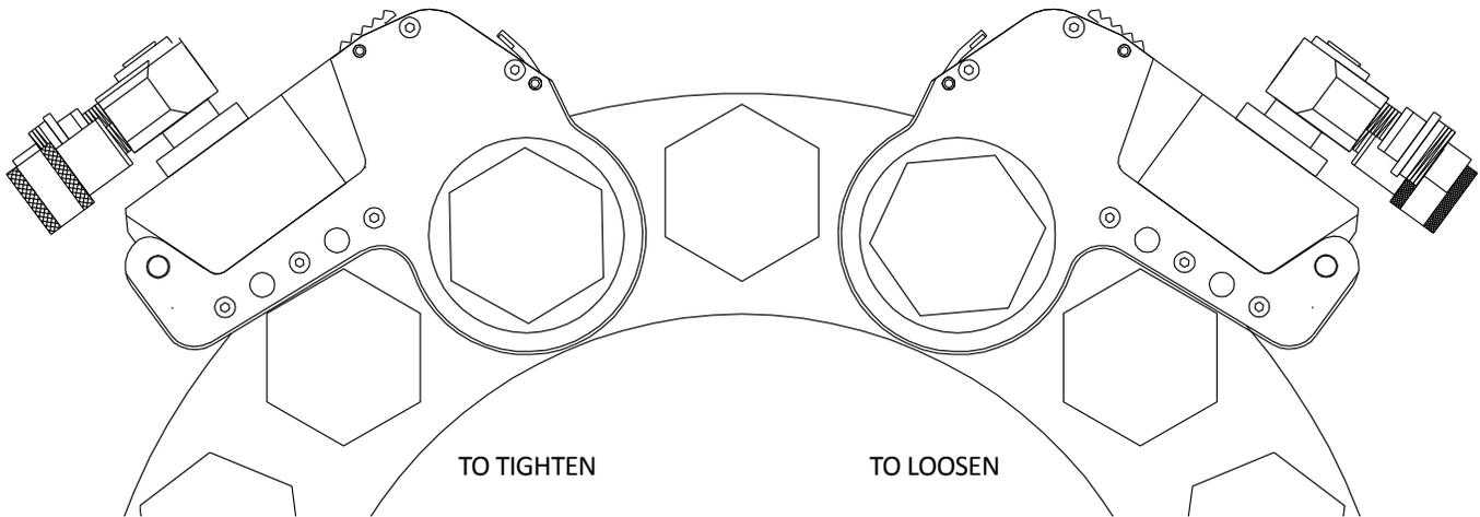
Positioning the tool determines whether the action will loosen or tighten the nut. Refer to above diagram for correct positioning. Assure the reaction area is firmly abutted against a stationary object (i.e. adjacent nut or flange) as illustrated.
