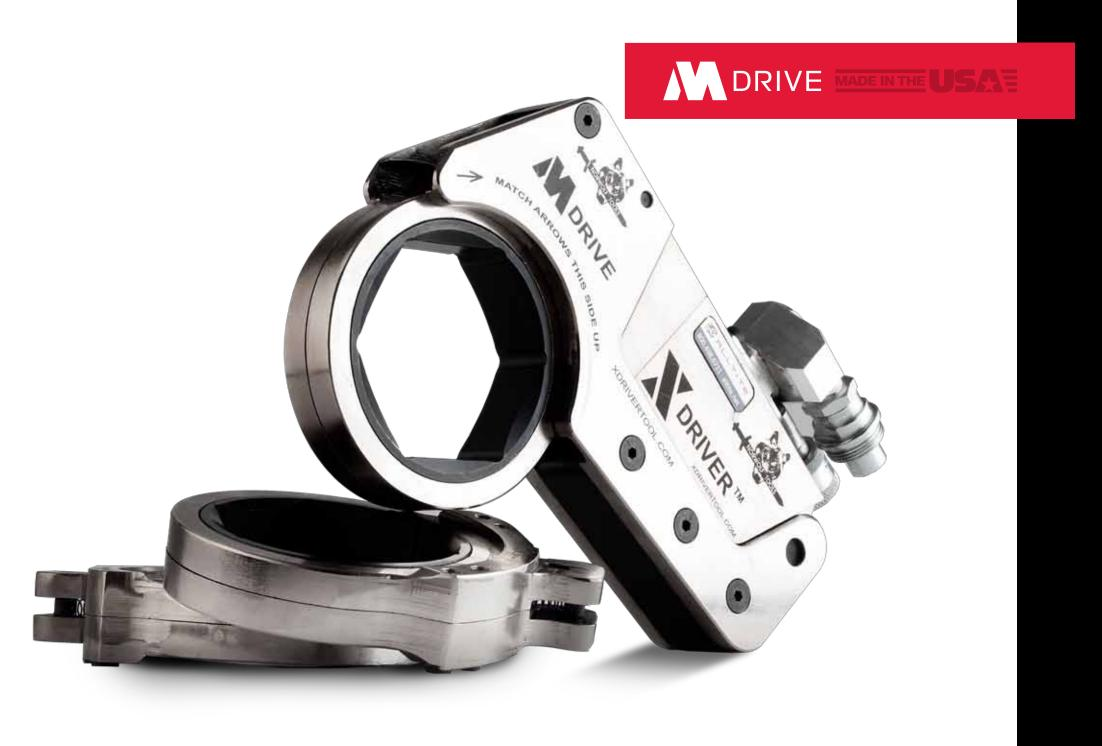
The M Drive is a special application tool for hyper-low clearance applications like BOP's. It has no holding pawl, is lightning fast and is the flattest drive width in the X Driver family. There are no roll pins. A longer lever arm allows for a 40 degree stroke, which is what gives the hex link it's amazing speed. The M Drive is specifically made for the tightest BOP applications (such as a 7" 10m) where no others can fit.
