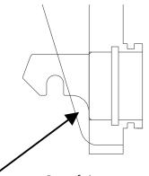
Base of piston must be within 1/16" of housing "B"
