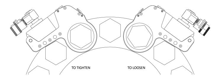
Positioning the tool determines whether the action will loosen or tighten the nut. Refer to above diagram for correct positioning. Assure the reaction area is firmly abutted against a stationary object (i.e. adjacent nut or flange) as illustrated.
